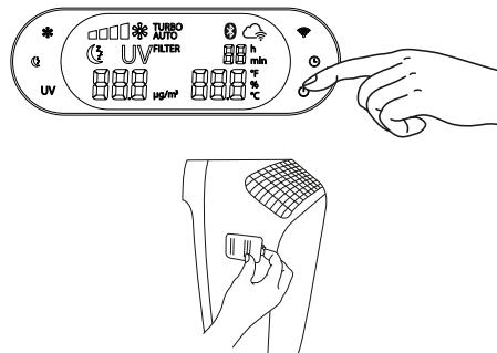
6. Insert the mains plug into the socket. Ensure that the cable does not pose a trip hazard. Press the ON/OFF button. Now open the flap on the side of the device housing. A button is located here to set the operating hour counter to 0.
