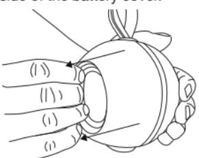
3. Now pull the battery out of the device and disconnect the battery from the device using the plug connection.
