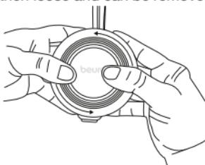
2. Then loosen the housing shell on the side of the battery cover.
