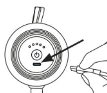
3. Connect the USB-C cable to a mains plug (not included in delivery). Insert
