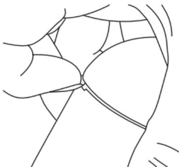
2. Insert both batteries into the battery compartment according to the specified polarity (+/-).
